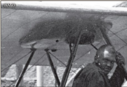
Gravity fuel tank (A14) detail from hexagon camouflaged AEG G.IV 588/17. Note the fairing over the fuel gauges (A9).
