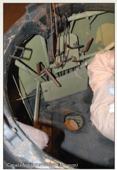
^ Although many small details are missing this is a good reference photo of the bomb release toggle and lever arrangement from AEG G.IV 574/18.
