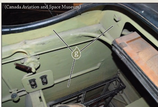
Bomb rack and crawl space beside the starboard fuel tank.
