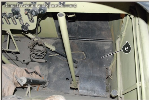
Cockpit floor with the commander's control stick installed.
