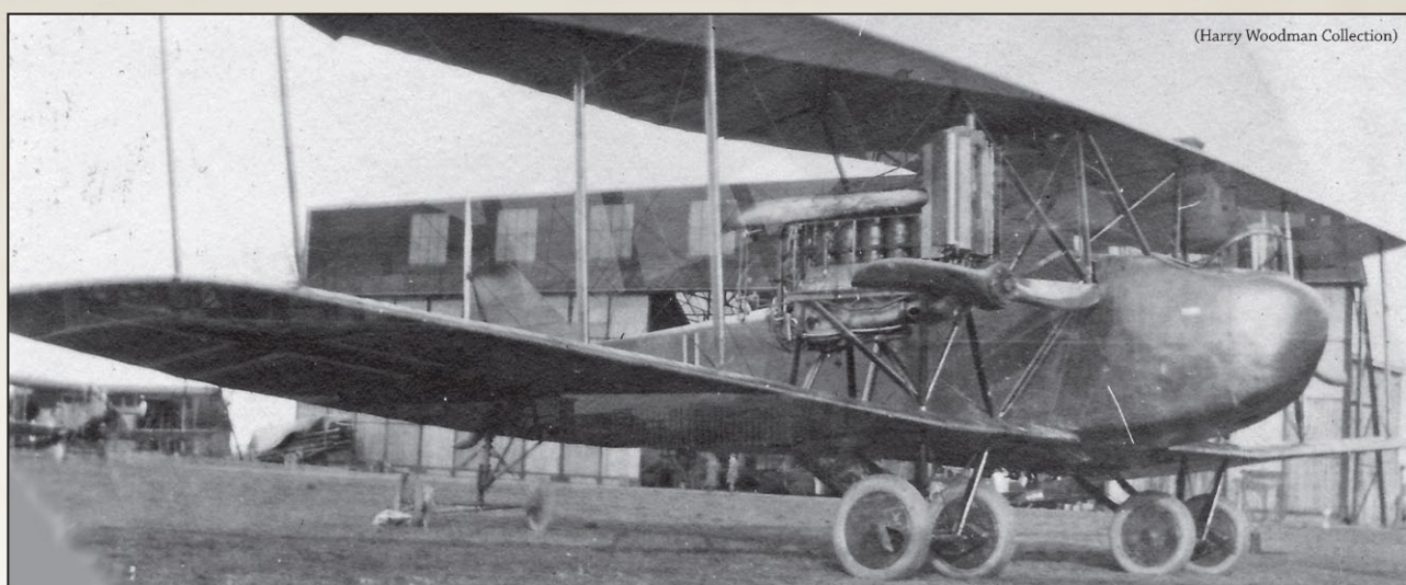
Starboard front \frac{3}{4} view. Note the commander's gun ring and distinctive bottom wing shape.
